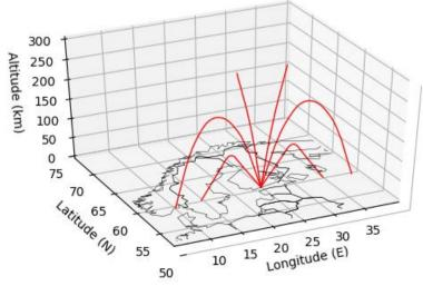
Left: Single hop skywave coverage map for various frequencies predicted by ray tracing
